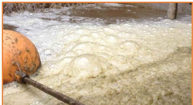
Effective foam control requires accurate data on foam behavioural parameters in real time. However, the effective and reliable measurement of foam thicknesses and foam-liquid interfaces presents a number of challenges. Traditional measurement techniques have been based on a range of existing level probe technologies 'adapted' for foam measurement. In most applications these tend to be inherently unreliable, inaccurate and adversely affected by process product build-up on the measuring probes.
